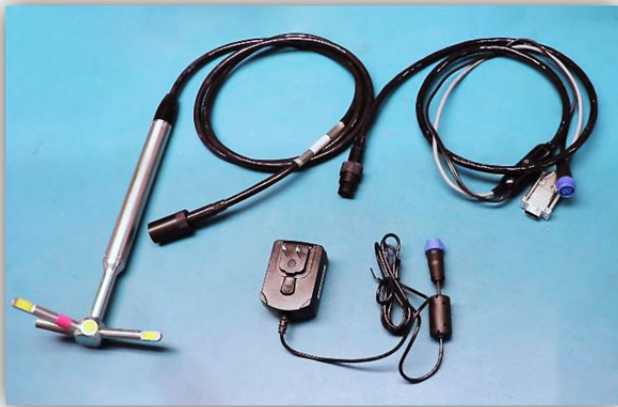
Figure 1. The FlowTracker2 Lab ADV probe assembly (left), along with its power and communications cable and power supply.
